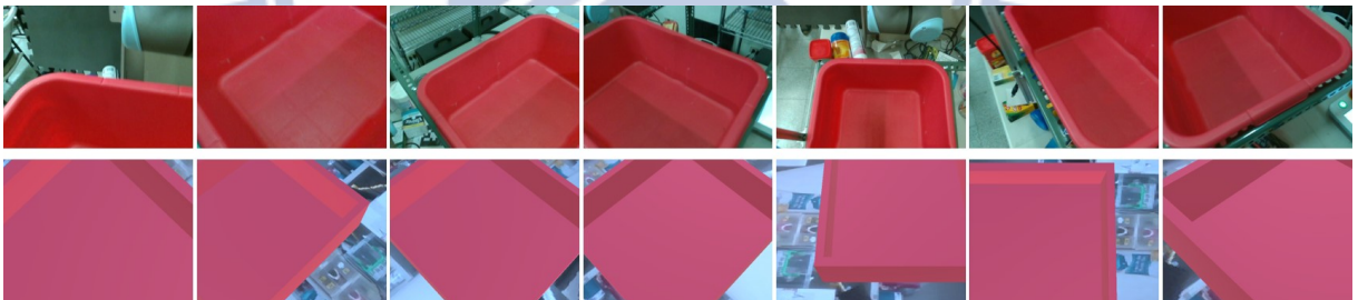
Figure 4.3: First row is the data in Real Tote Dataset, and the second row is the Unity box images in Unity Virtual Dataset.
